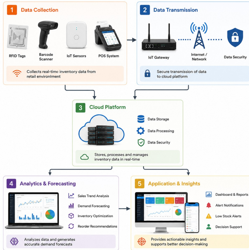
Figure 3. Proposed IoT-integrated smart inventory management framework for retail operations.
